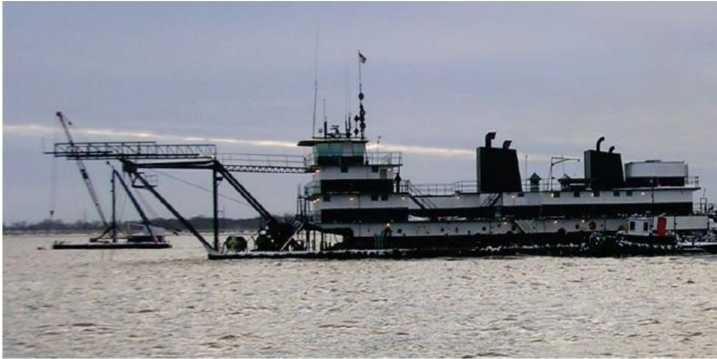
The Pullen is a 150-foot-long cutterhead-pipeline hydraulic dredge deployed by the Norfolk Dredging Company for New Pass and Longboat Pass Dredging and Beach Nourishment Projects.
